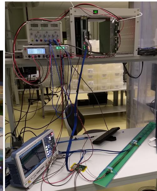
Followed identical ALICE IB QA test procedure, with a 8m SamTec cable!
