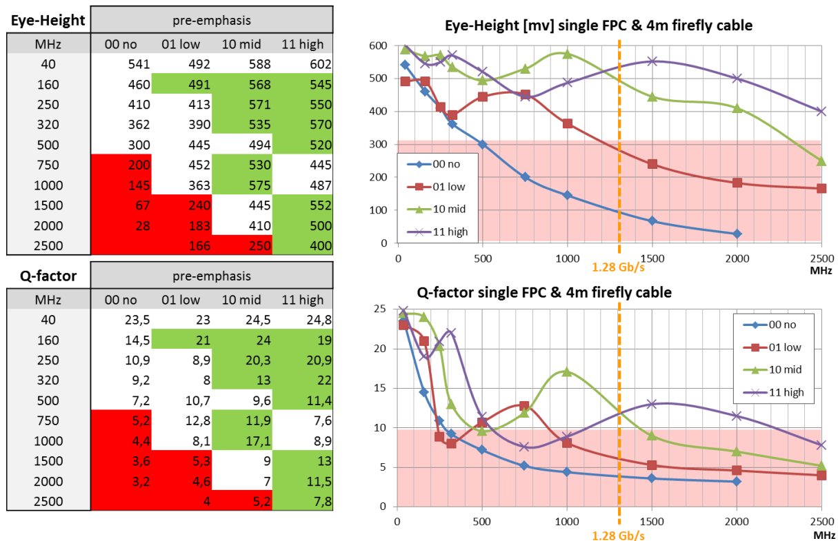
Figure 47 – Inner Layers configuration test mock-up measurements. 30 cm long FPC plus 4m AWG30 twinax cables.
