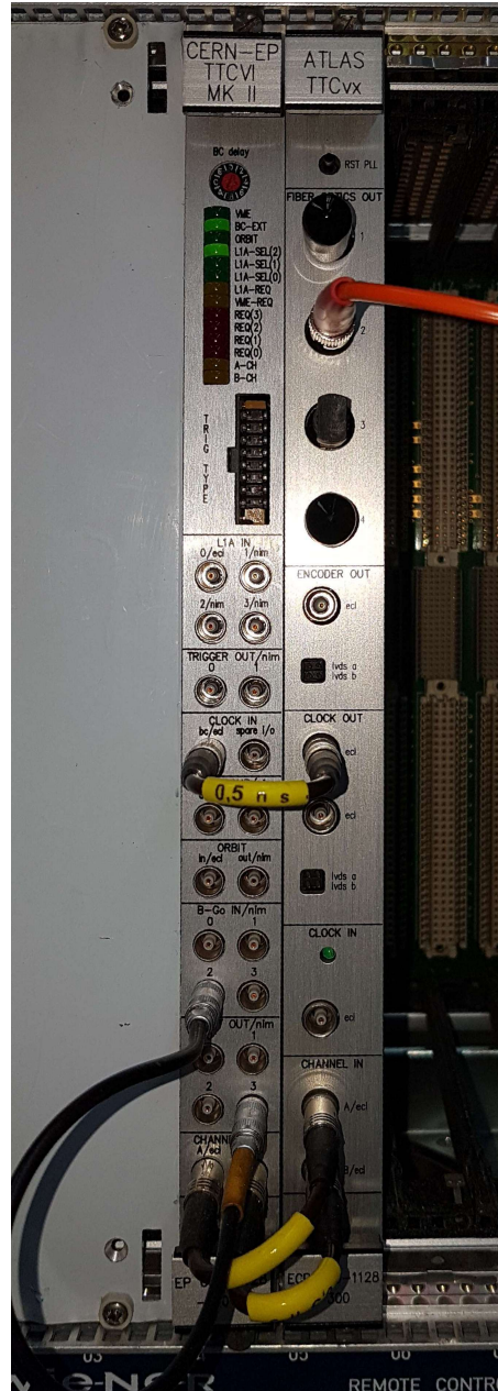
Figure 70: Image of cabled TTC system with B-channel connections
