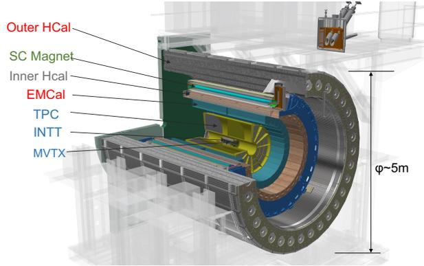
Fig. 1. A schematic view of the sPHENIX detector
