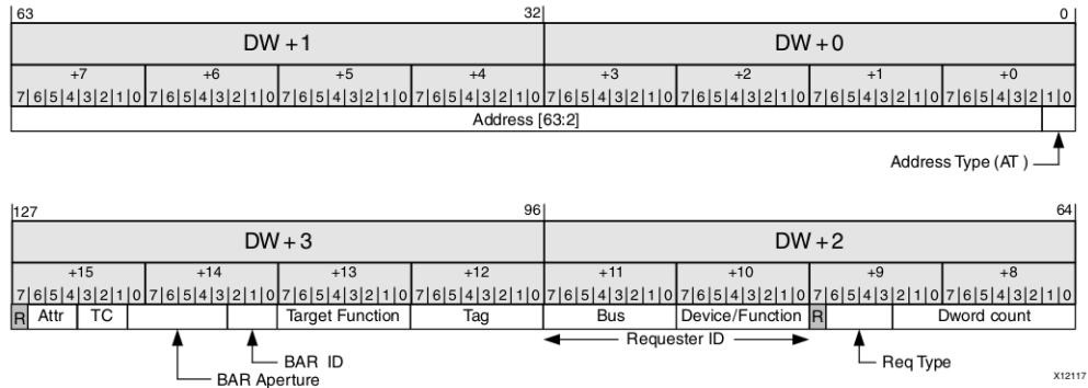
Figure 86: Completer Request Descriptor Format for Memory I/O
