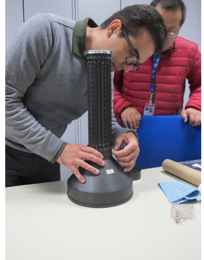
Inner tracker staves mounted to prototype support ends.
