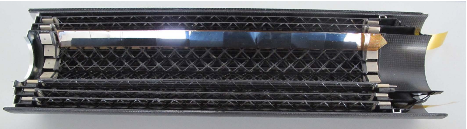
Prototype inner tracker half barrel layers showing staggered layer overlap to maintain continuous coverage in \phi
