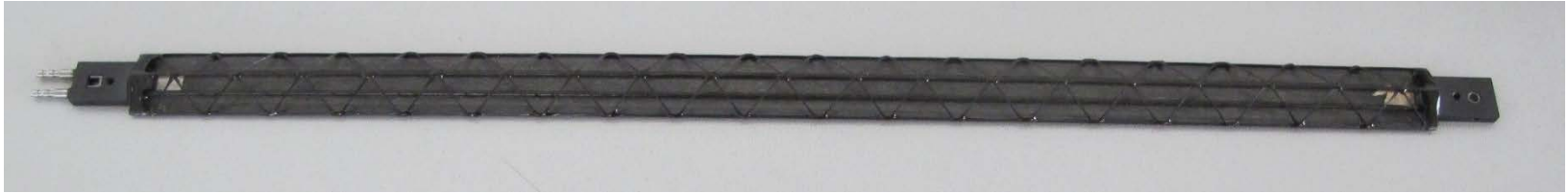
ALICE inner tracker production stave with cooling tubes and filament support
