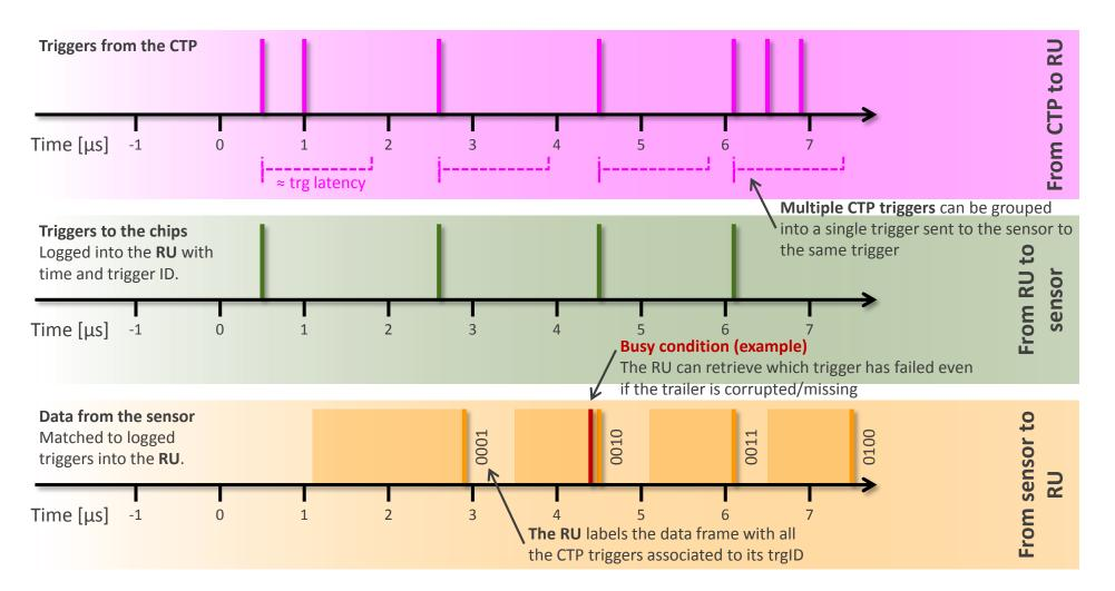
Triggers close in time re-record the same information, and the sensor can handle a minimum trigger spacing of about 1  $\mu$ s. The RU will therefore "filter" close-in-time ( $\approx < 1 \mu$ s) triggers. This also allows for the busy flag to be propagated to the readout unit before another trigger is issued (see next slide).
