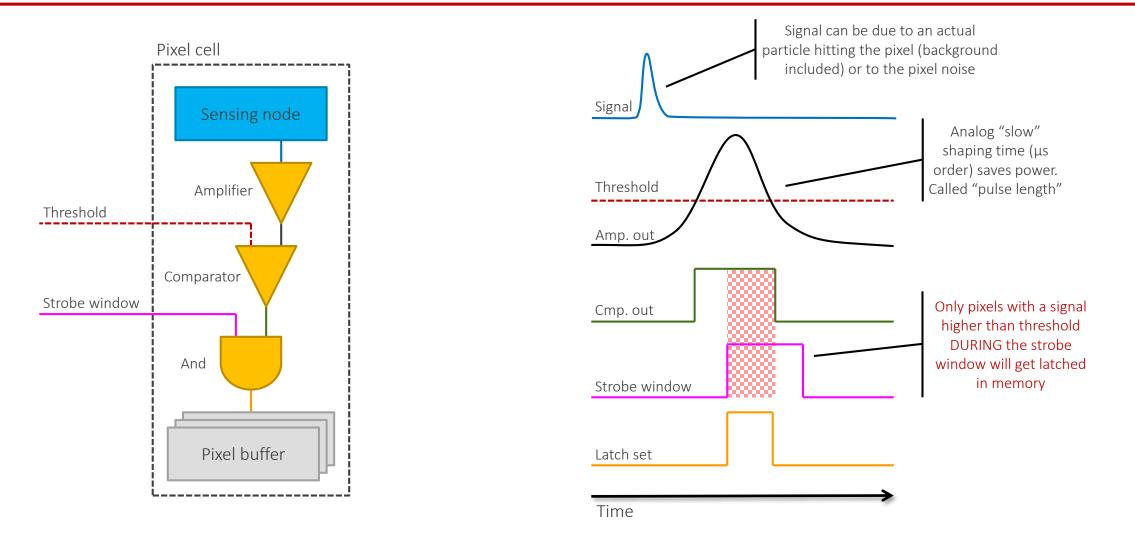
Slow shaping time acts as an analogue memory buffering the signal until the arrival of the trigger (time over threshold of about 5 µs on average). Signals above threshold during the strobe window are latched into one of the pixel memory buffers.
