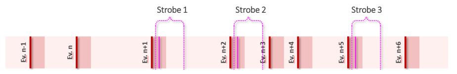
*Continuous mode*: Pixels are latched using long, periodic strobe windows with short inter-strobe periods (≈100 ns) to initiate read out.
