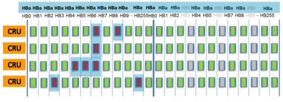
By sending some Heart Beat **Reject** triggers the CTP (resulting suppressed HBF grey rectangles) can effectively throttle down the acquisition bandwidth, improving the likeliness of having aligned data frames.
