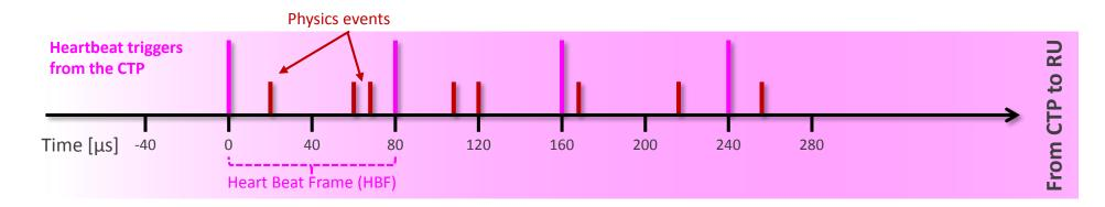
The CTP also collects a <u>busy condition</u> from each Common Readout Unit for each HBF. In case of excessive busy occurrence in one or more detectors, the CTP will <u>throttle down</u> the overall acquisition speed by sending a special Frame Suppress trigger.
