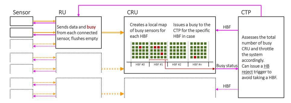
The CRUs connected to the ITS have all the information to <u>internally compute a "busy map" of all the sensors it is</u> <u>connected with</u> (other detectors CRUs will only check their own internal buffer). They can individually assert a busy condition to the CTP.
