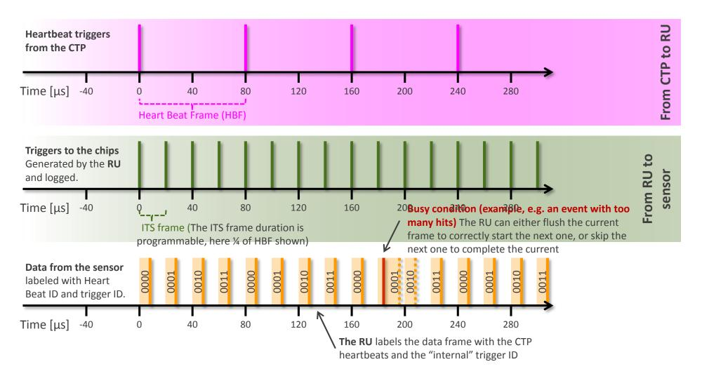
The sensor has an embedded (programmable) trigger generator, *but we will instead issue triggers at a constant frequency from the Readout Unit* for continuous mode operation to ensure more flexibility in managing busy and potential error conditions, as well as for implementing <u>local frame throttling/suppression schemes as needed</u>.
