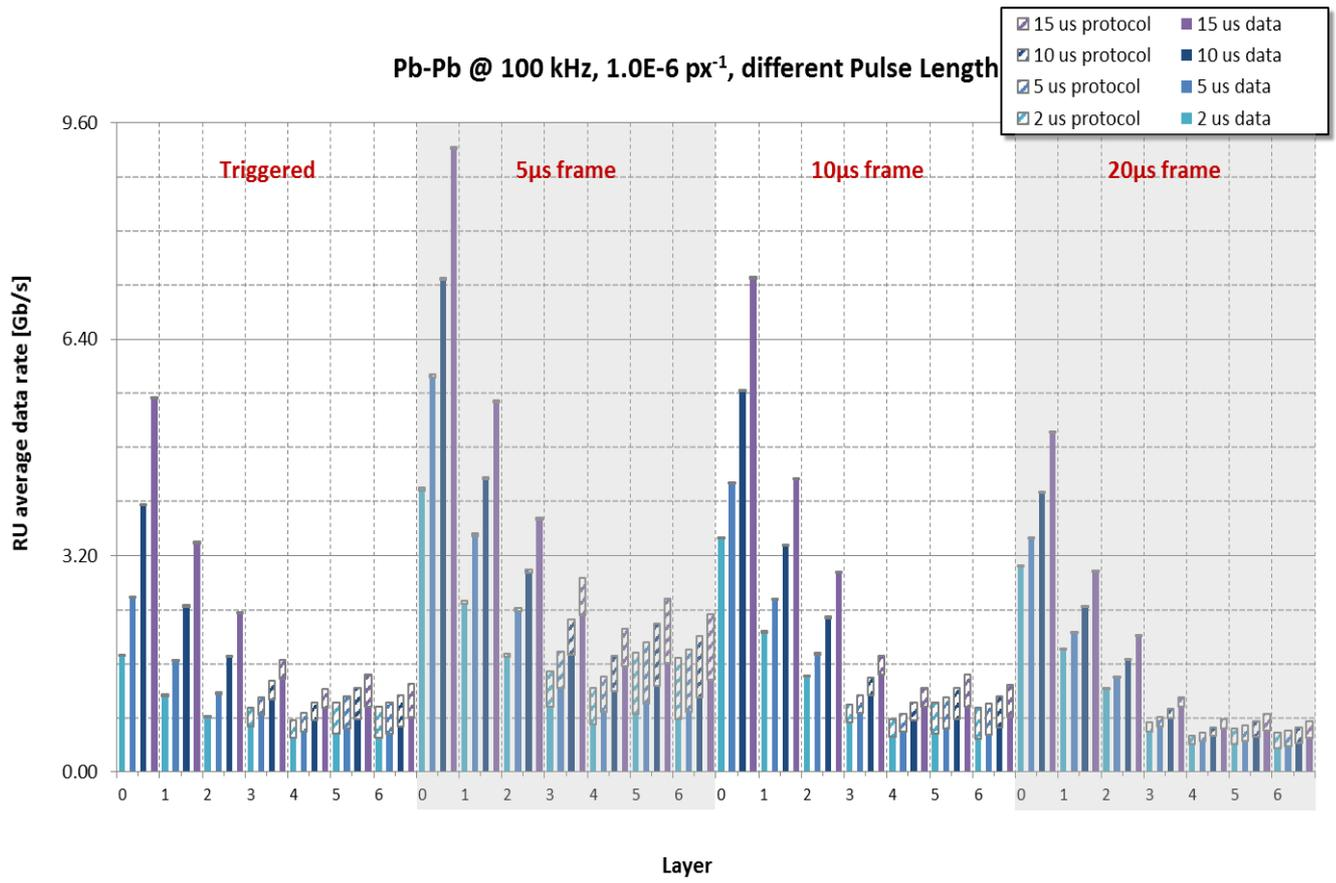
Figure 6 – Pb-Pb @ 100 kHz, noise 10<sup>-6</sup> px<sup>-1</sup>, different shaping times, data and protocol breakdown.
