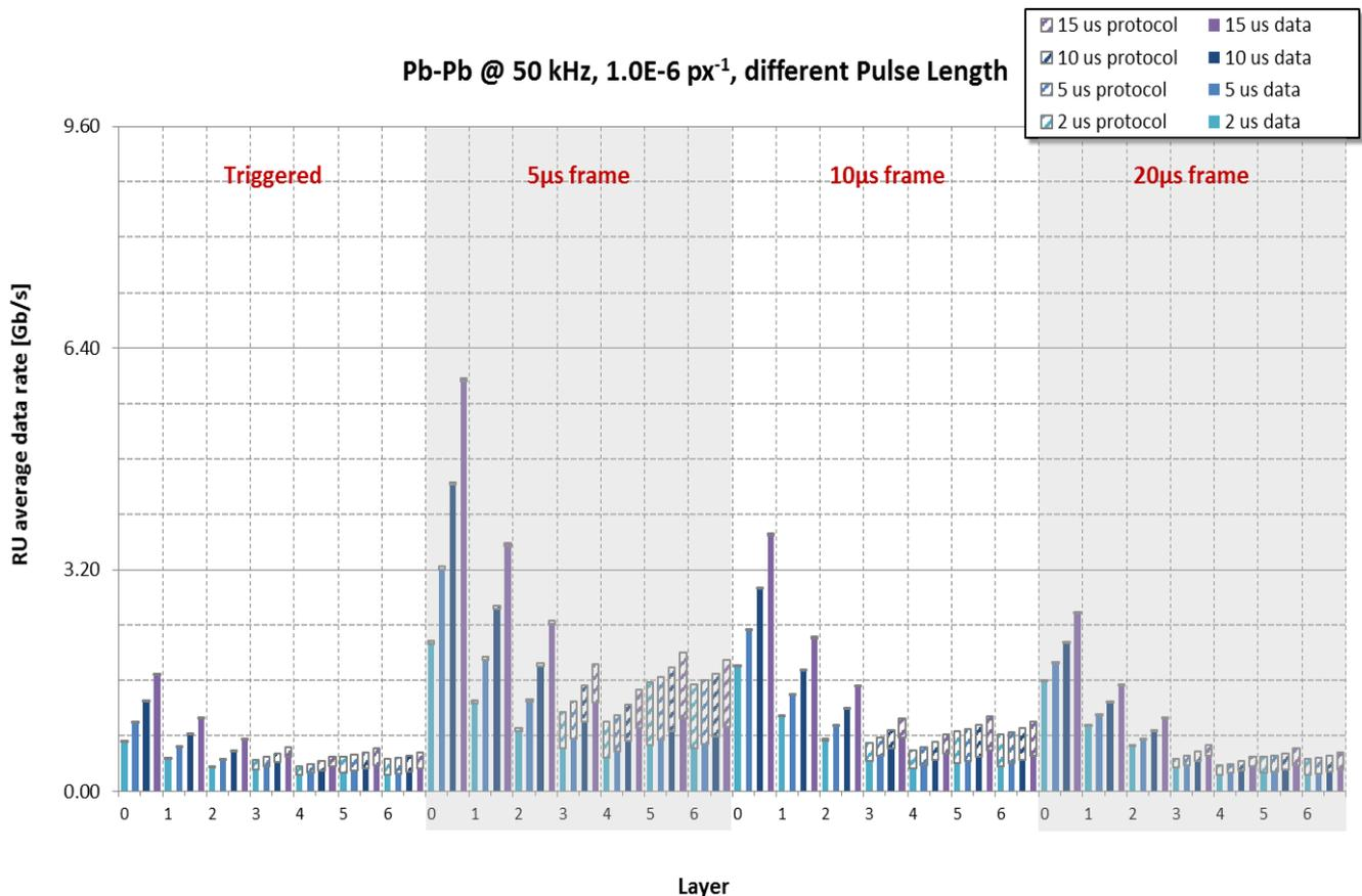
Figure 5 – Pb-Pb @ 50 kHz, noise  $10^{-6}$  px<sup>-1</sup>, different shaping times, data and protocol breakdown.
