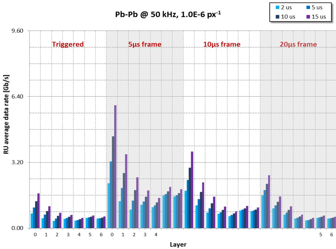
Figure 1 – Pb-Pb @ 50 kHz per RU bandwidth for different shaping times, noise of 10<sup>-6</sup> px<sup>-1</sup>.
