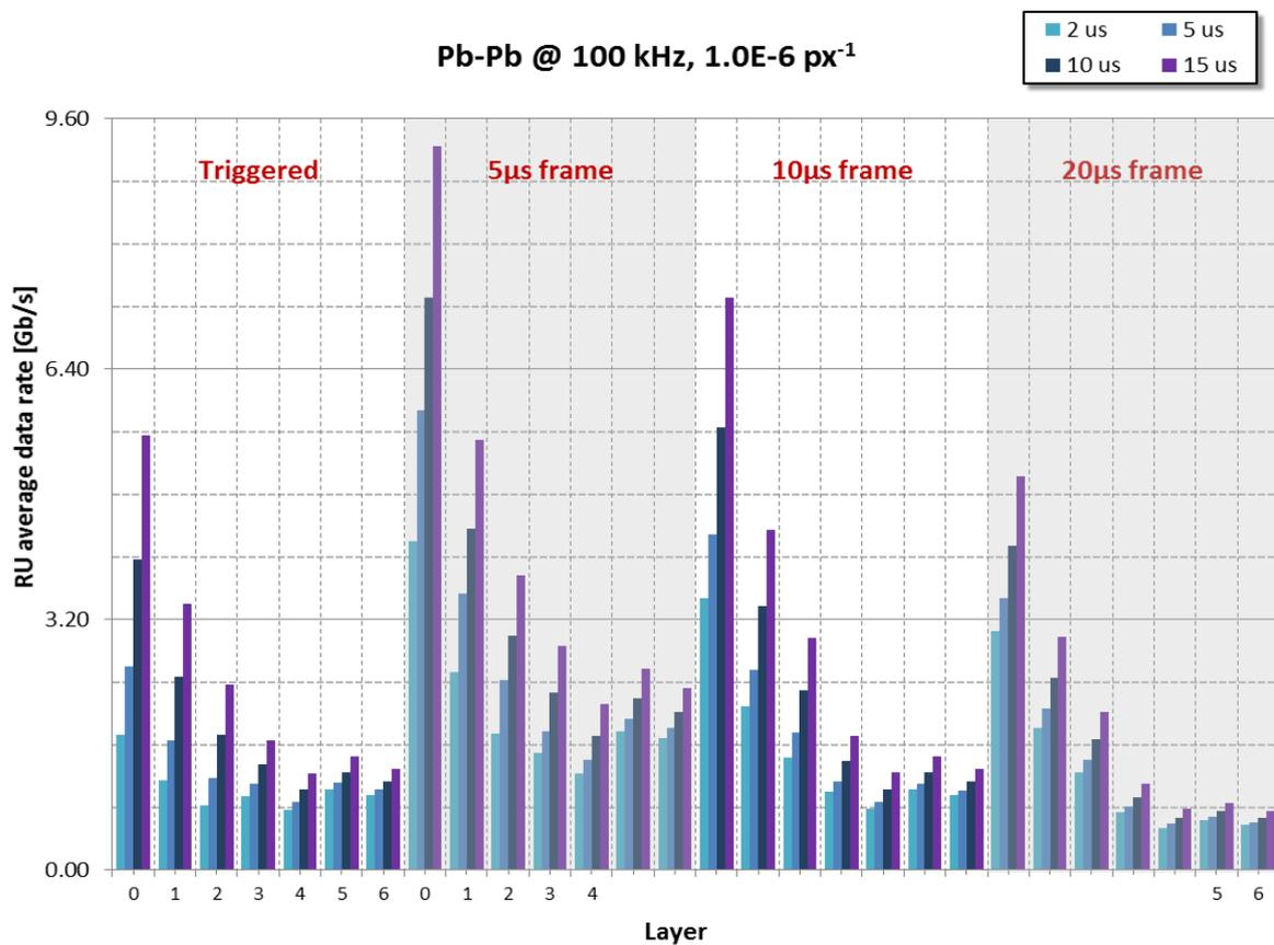
Figure 2 – Pb-Pb @ 100 kHz per RU bandwidth for different shaping times, noise of 10<sup>-6</sup> px<sup>-1</sup>.
