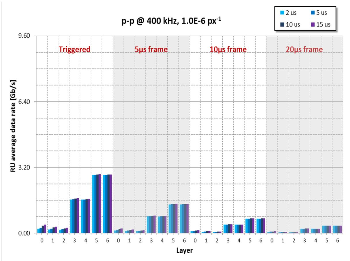
Figure 3 – p-p @ 400 kHz per RU bandwidth for different shaping times, noise of 10<sup>-6</sup> px<sup>-1</sup>.
