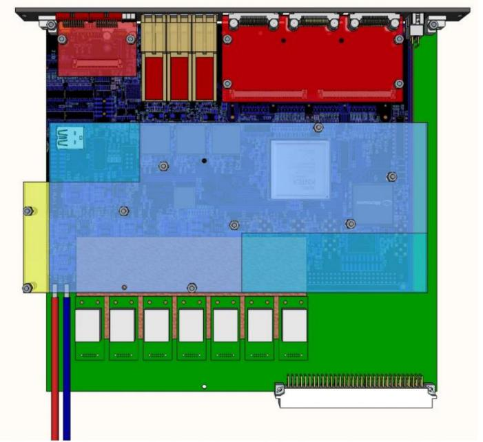
It could be an opion to replace the single 208-pin samtec QFS/QMS-style connector with 2 ERF8/ERM8 connectors. T.B.I.
