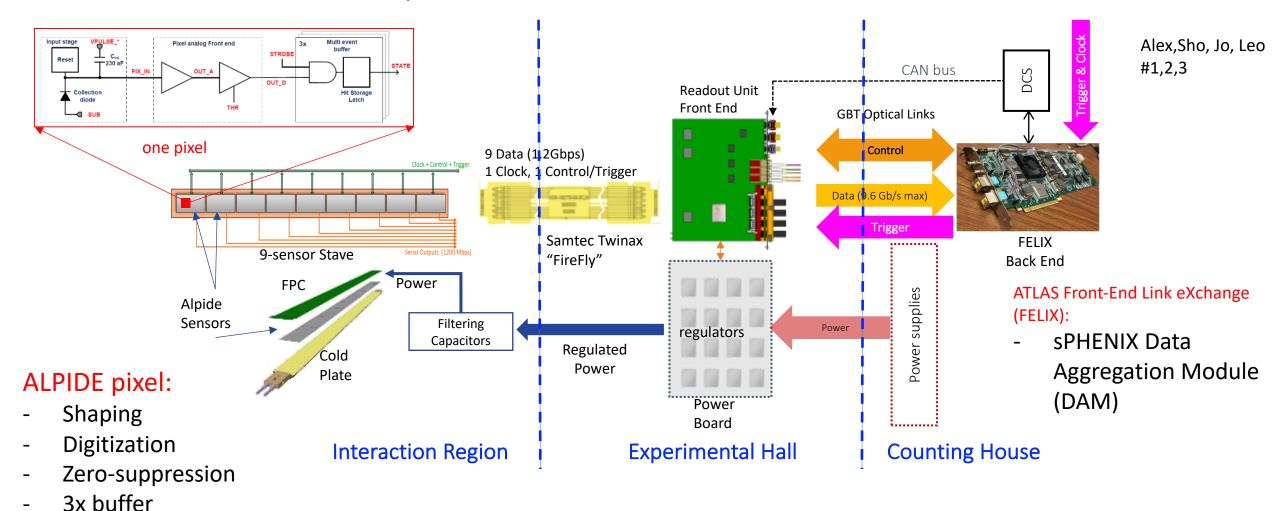
MVTX Detector Electronics consists of three parts
