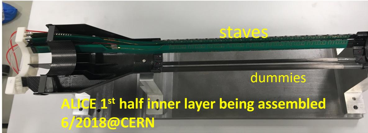
Precision positioning and installation of staves on end-wheels
