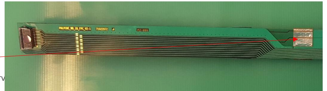
The PWR extension is connected to the FPC by iron soldering and wings are cut.
