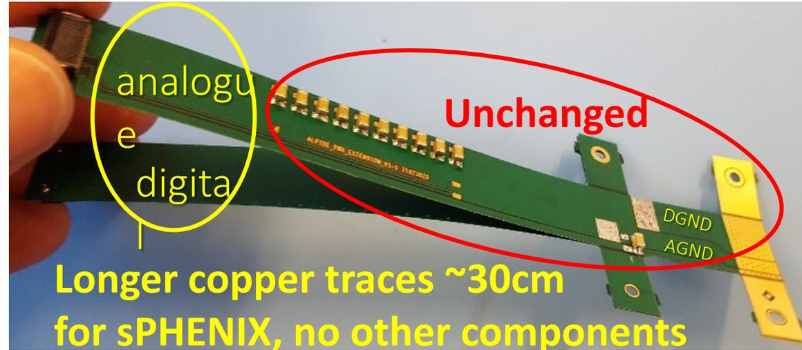
The two flexes are connected together, AVDD is transferred from top to bottom
