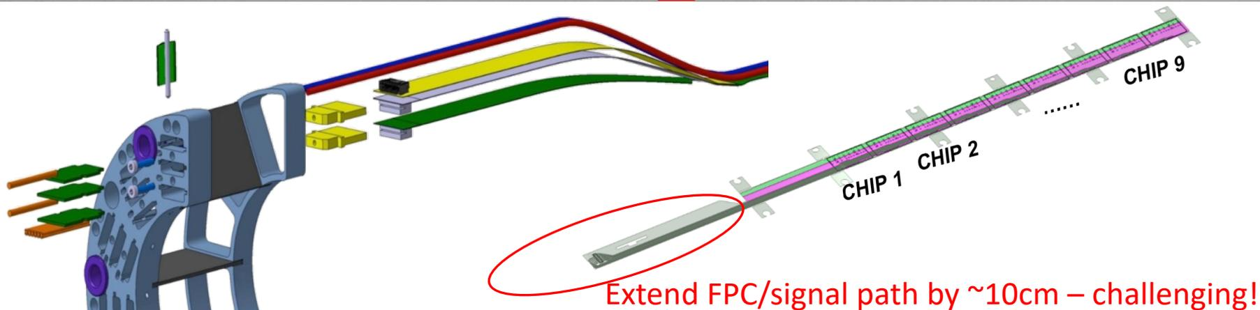
The 9 silicon chips are read out in parallel: each chip sends its data stream to the end of Stave by a dedicated differential pair, 100  $\mu\text{m}$  wide. Two additional differential pairs distribute the clock and configuration signals.
