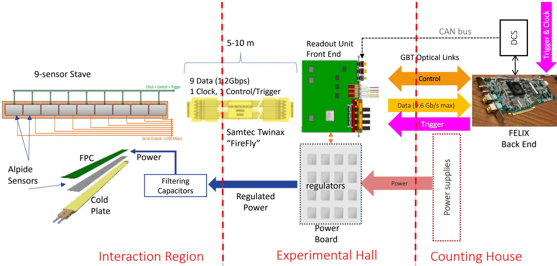
MVTX Detector Electronics consists of three parts
