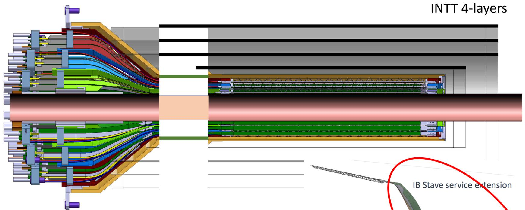
**MVTX:** Extend cables to move the conical structure further out in z-direction
