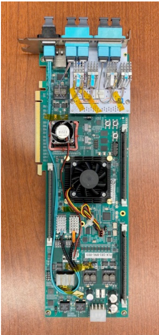
Assembled 24ch FLX-181 with 25 Gbps FireFly FMC+
