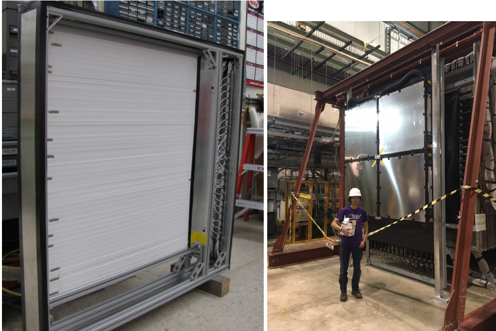
Figure 2: Left: One of eight hodoscope quadrants built for the 2017 displaced di-muon trigger upgrade. Right: The downstream hodoscope after installation.
