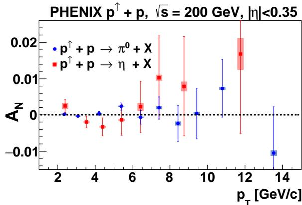
FIG. 4. Comparison of the  $\pi^0$  and  $\eta$  meson asymmetries measured at  $|\eta| < 0.35$  in  $p^\uparrow + p$  collisions at  $\sqrt{s} = 200$  GeV. An additional scale uncertainty of 3.4% due to the polarization uncertainty is not shown.
