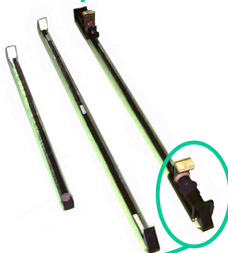
Slat: Plastic scintillator w. 2 PMT's
