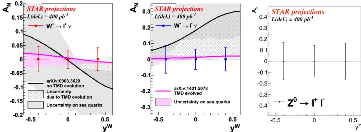
Figure 2-4: The projected uncertainties for transverse single-spin asymmetries of  $W^\pm$  and  $Z^0$  bosons as functions of rapidity for a delivered integrated luminosity of  $400\text{pb}^{-1}$  and an average beam polarization of 55%. The solid light gray and pink bands represent the uncertainty on the KQ [44] and EIKV [41] model, respectively, due to the unknown
