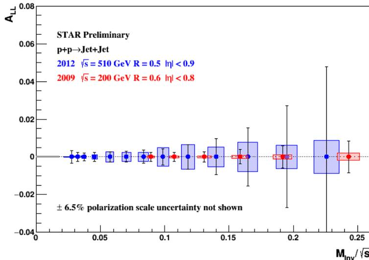
Figure 3-1: The projected accuracy for the di-jet double spin asymmetry  $A_{LL}$  versus  $M_{inv}/\sqrt{s}$  of the pair for mid-rapidity p+p collisions at  $\sqrt{s} = 200$  (red) GeV and  $\sqrt{s} = 510$  (blue) GeV. The recorded luminosity of both data sets is  $21.2 \text{ pb}^{-1}$  for 2009 and  $60 \text{ pb}^{-1}$  for 2012.
