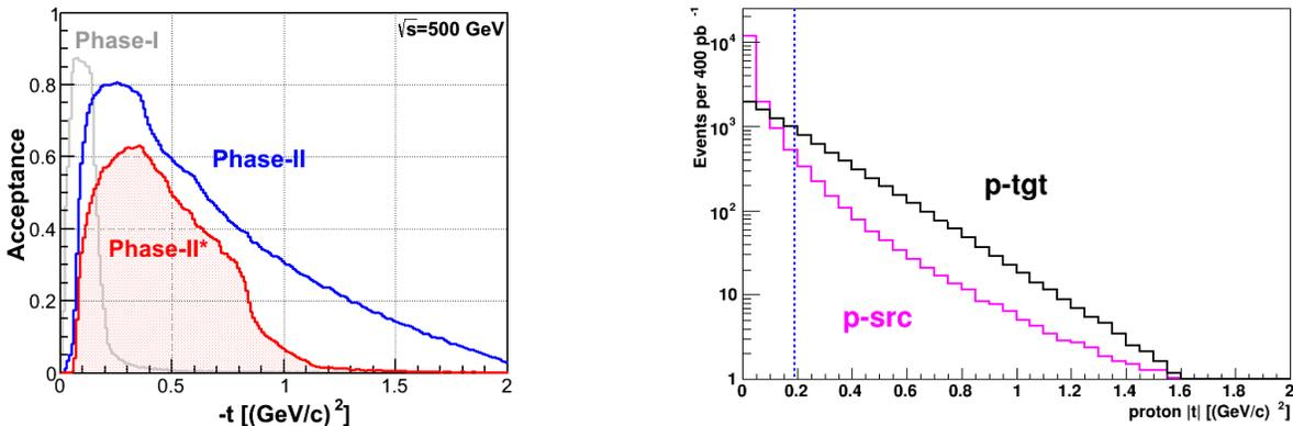
Figure 2-17: (left) Acceptance of protons in exclusive  $p+p$  scattering at  $\sqrt{s} = 500$  GeV as function of  $t$  for a possible future upgrade (blue) and the STAR set up since 2015 (PHASE-II\*) (red) configuration. The acceptance for the original STAR Phase-I setup is also shown (grey). (right) The  $t$  spectrum of the proton emitting the photon (pink) as well as the one from the scattered proton (black).
