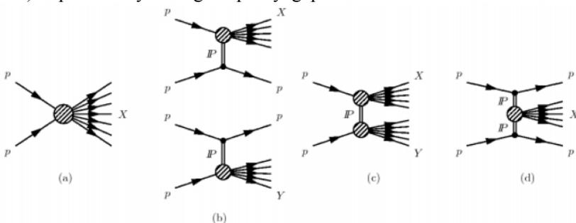
Figure 2-15: Schematic diagrams of (a) nondiffractive,  $pp \rightarrow X$ , (b) singly diffractive,  $pp \rightarrow Xp$  or  $pp \rightarrow pY$ , (c) doubly diffractive,  $pp \rightarrow XY$ , and (d) centrally diffracted,  $pp \rightarrow pXp$ , events.
