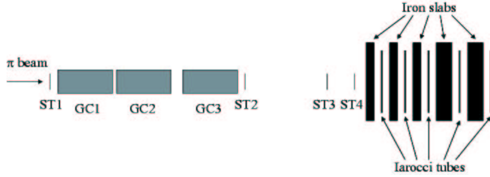
Figure 2.24 Setup for the MuID beam test carried out at KEK-PS. Four scintillation counters (ST1 to ST4) define the beam. Three gaseous Čerenkov counters (GC1 to GC3) identify pions and muons.
