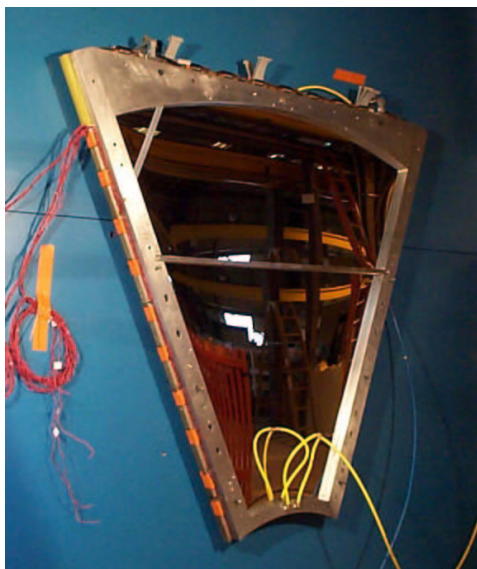
Figure 2.13 A photograph of a MuTr station-2 octant. A cathode plane is made of etched 25- \mu\text{m} copper coated mylar foils.
