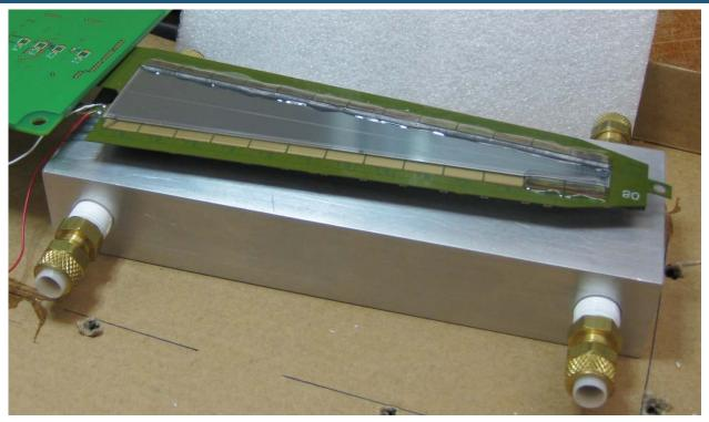
Thermal measurements made on 15 chip wedge assembly, powered LVDS at 390. ma, 2.6 V = 528.1 microwatts per channel. Measured 29 ° C to 36 ° C along 13 chips, no coolant or contact with Aluminum plate. Temperature dropped 2 ° C when spacers in contact with Aluminum @ 23 ° C. Sensor deflection and temperature differential across the wedge vary linearly with chip power.
