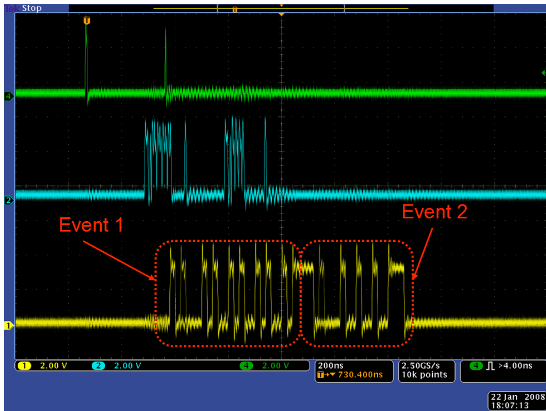
Figure 18 Scope screenshot of a two events being outputted from two consecutive clocks. Green trace show transfer of the data to sub-buffers, blue – write enable for output buffer.
