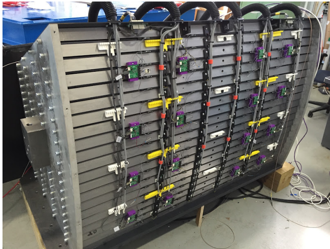
Outer HCAL prototype with assembled steel plates and readout electronics
