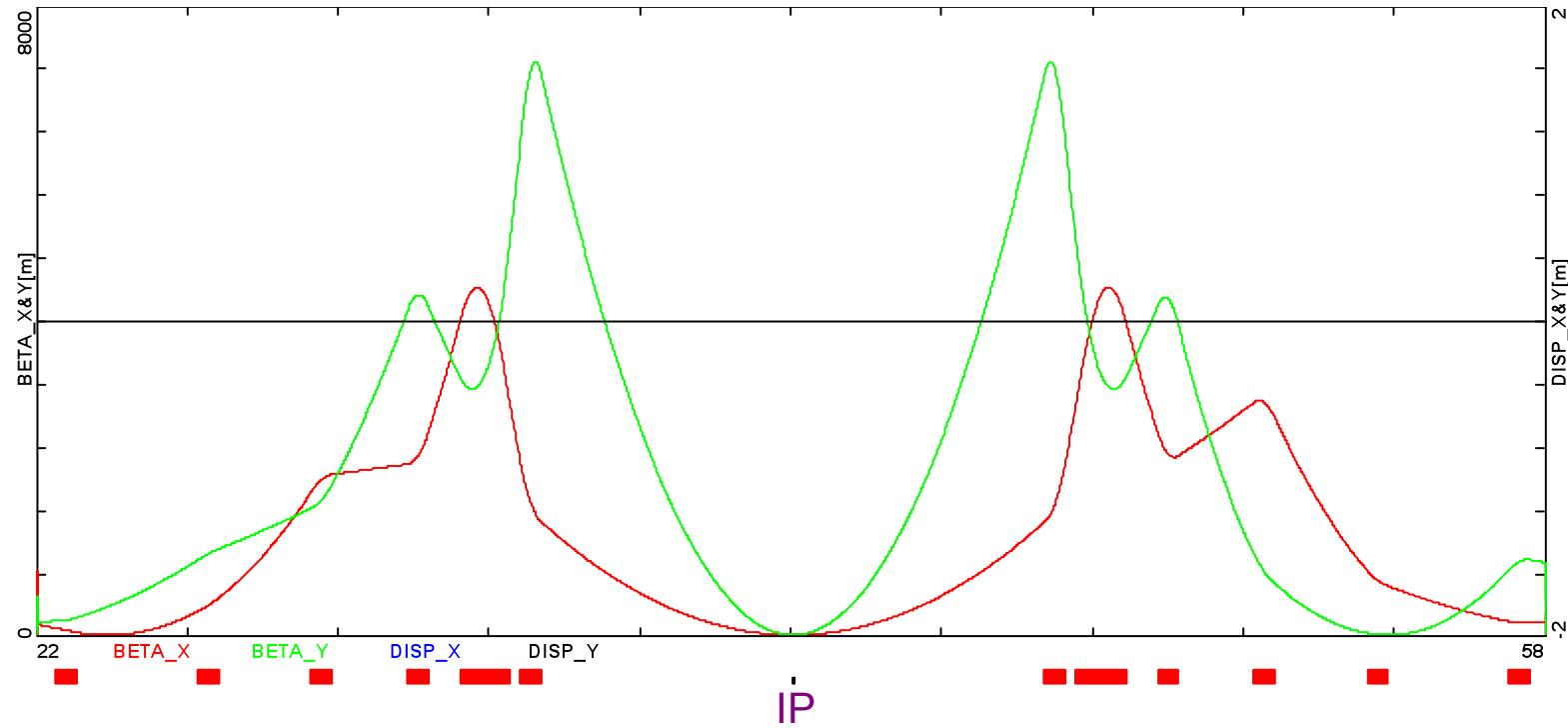
$$\zeta_{x,y}^{IR} \simeq -\frac{1}{4\pi} \sum_i \beta_{x,y}^i \int g_0^i ds = -\frac{1}{4\pi} \sum_i \beta_{x,y}^i k_1^i \quad k_1 = \frac{1}{B\rho} \int \frac{\partial B_y}{\partial x} dl = \frac{e}{pc} \int \frac{\partial B_y}{\partial x} dl [m^{-1}]$$
