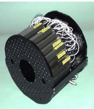
Beam-beam counter (BBC) |\eta|=3\sim 4 64pmts in each BBC charged particles
