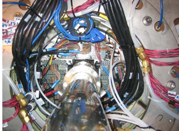
(c) Photograph of the MPC North Arm after installation in the North Muon Arm piston.
