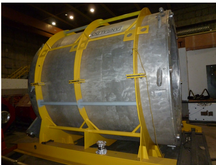
Figure 3.2: The BaBar solenoid in its transfer frame for shipping at SLAC in May, 2013.
