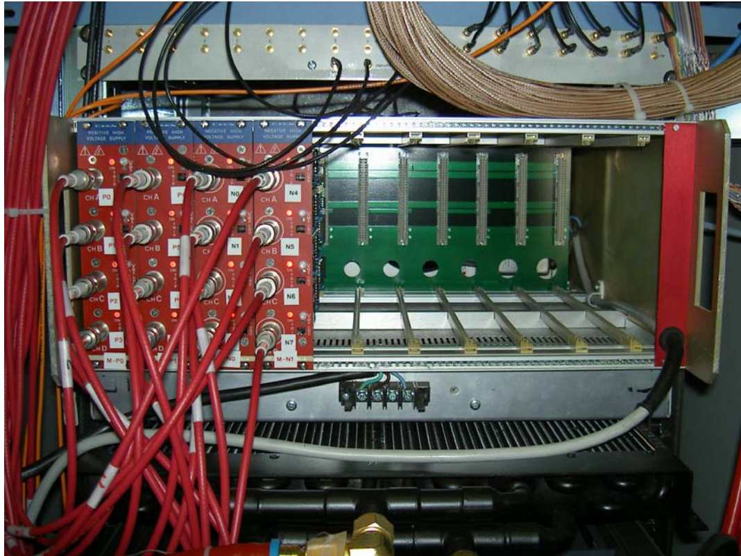
Figure 47. CEAN SY127 mainframe and A631P and A631N modules in RUN 5. The same configuration will be installed on each side of the TOF.W detector.
