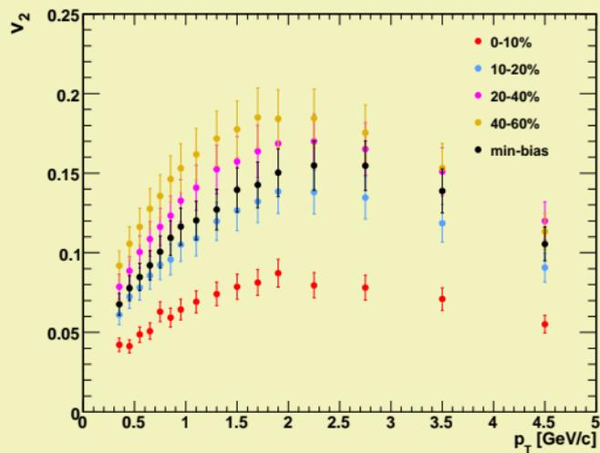
$v_2$  of inclusive electrons measured using the event plane from the new RXPN detector.
