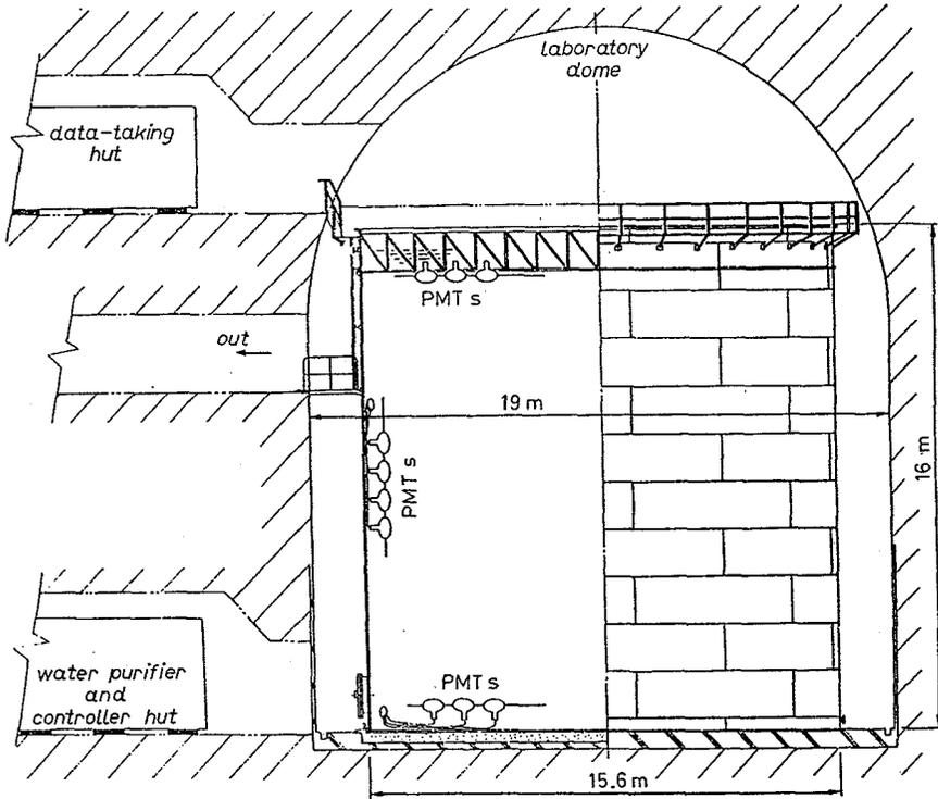
Fig. 9.4. - A schematic view of the 3000 m<sup>3</sup> water tank and phototube support system of the Kamioka proton decay experiment [84K3].
