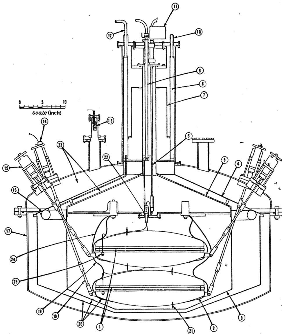
Fig. 11.2. - The Chicago-Fermilab-Michigan prototype detector. The scale is set by the diameter of the loops, which is two feet [83F4].
