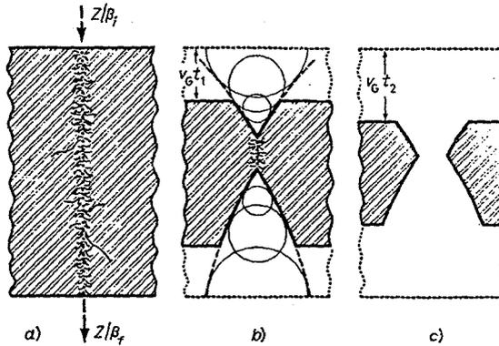
Fig. 3.8. — Track-etching technique for particle identification: a) sketch showing dense core of radiation-damaged material and delta-rays; b) development of conical etch pits at the intersection of the trajectory with the surface; c) development of a hole after prolonged etching [82B2].
