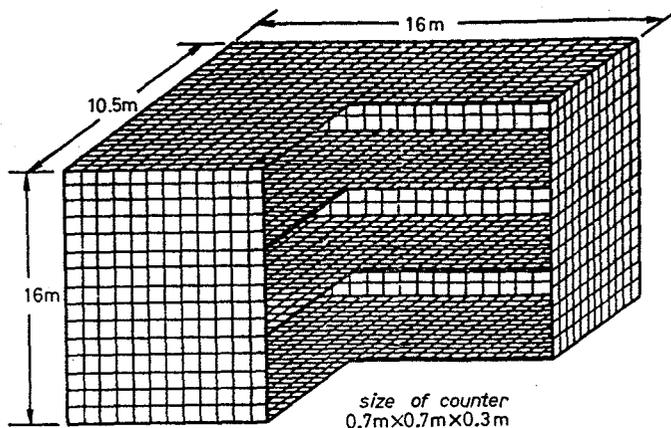
Fig. 8.9. – Lay-out of the Baksan mountain (USSR) liquid-scintillator detector [82A1].
