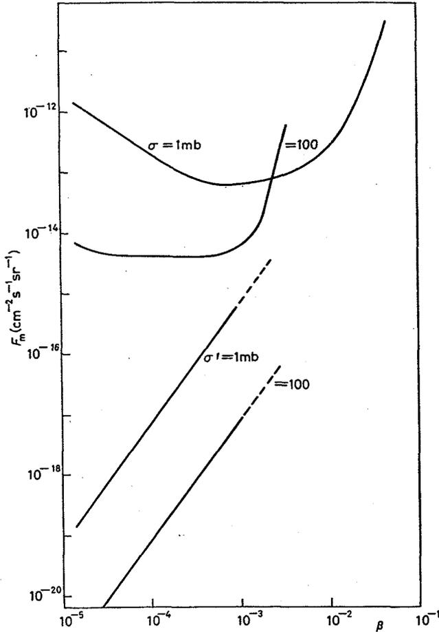
Fig. 9.5. - Upper limits (90% c.l.) on the monopole flux vs. monopole velocity for the multiple catalysis of proton decay in the Kamioka water Čerenkov detector for several values of the catalysis cross-section [84K3]. Also shown are upper limits from solar neutrinos (see text).
