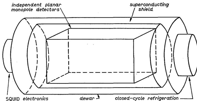
Fig. 11.1. - Sketch of the proposed IBM superconducting induction lay-out.
