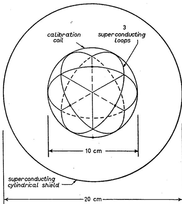
Fig. 8.3. - Schematic view of the Stanford three-loop superconducting induction detector [83C3].
