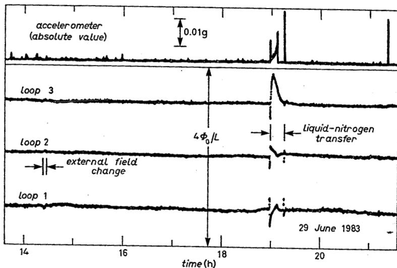
Fig. 8.6. - Chart recording of the three loops and of the accelerometer of the Stanford induction detector [83C3]. Notice the disturbances generated at the time of the liquid-nitrogen transfer in the outer cryostat.
