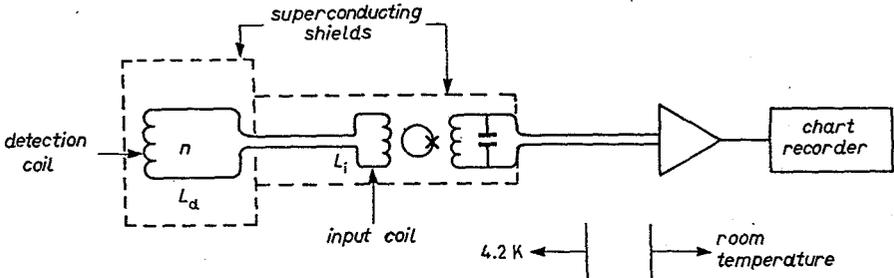
Fig. 8.1. – Schematic diagram of a superconducting induction detector for magnetic monopoles [83T2]. The detection coil is coupled to an input coil for the SQUID device, whose output is amplified and sent to a chart recorder.
