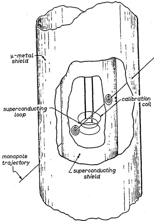
Fig. 8.2. - Schematic view of the first Stanford superconducting loop [82C1]. Notice the magnetic shieldings (superconducting and mu-metal) and the two trapped magnetic fluxes in the superconducting shields.
