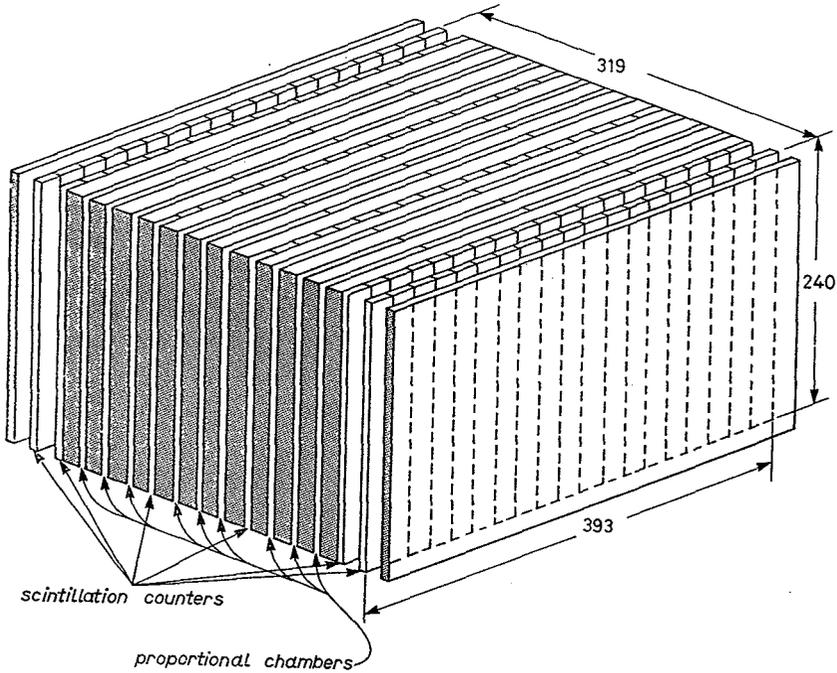
Fig. 8.10. - Lay-out of a Tokyo detector, which used the Drell and Penning effects (see text) [83A7]. Units in cm,
