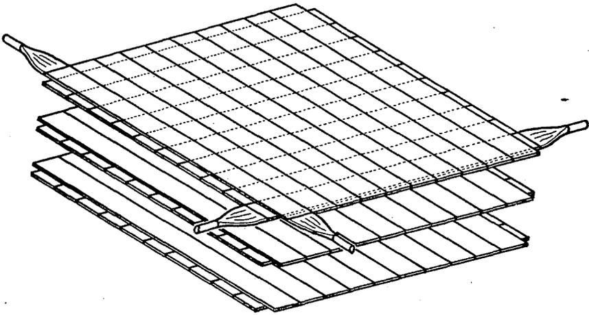
Fig. 8.8. - Lay-out of the Tokyo-Kamioka mine monopole detector [83M1], with 6 planes of counter hodoscopes.
