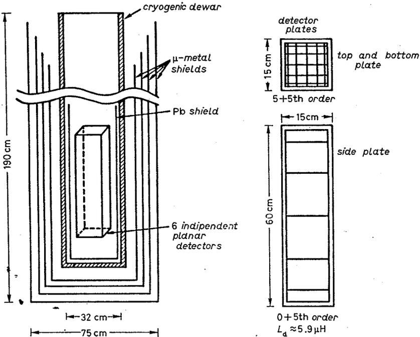
Fig. 8.5. - The present IBM detector. Six planar gradiometers placed on the faces of a parallelepiped are independently monitored by six SQUIDS (not shown). This provides a geometry with 100% coincident detection [83C6, 83T3].
