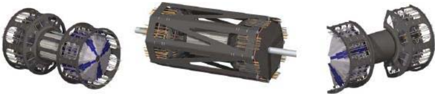
Figure 4.2-1: Various PHENIX Tracker Support Structure Concepts Studied for Structural Stiffness.
