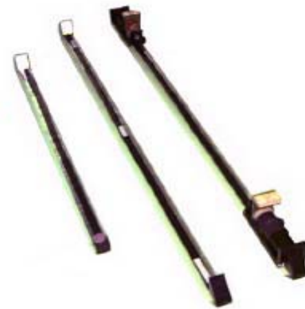
Slat; Plastic rod w. 2 PMT's
