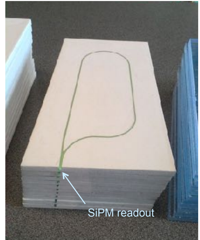
Polystyrene scintillating tiles (7 mm) with WLS fiber (1 mm). One SiPM reads out both ends of fiber. SiPMs from 5 tiles summed into 1 tower
