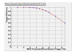
RICH J/Ψ trigger efficiency as a function of threshold on number of photoelectrons per tile
