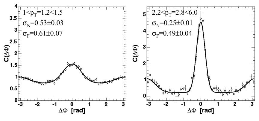
$Fit = const + Gauss(0) + Gauss(\pm \pi)$
