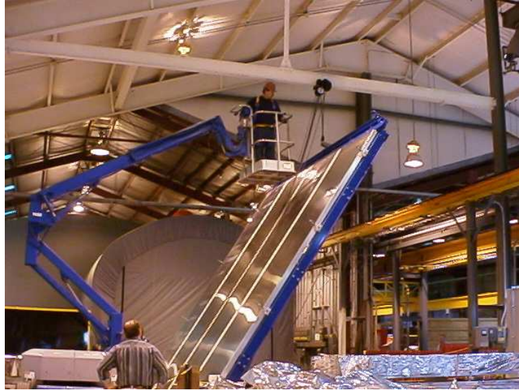
Figure 2.21: Muon identifier panel being flipped over during construction.
