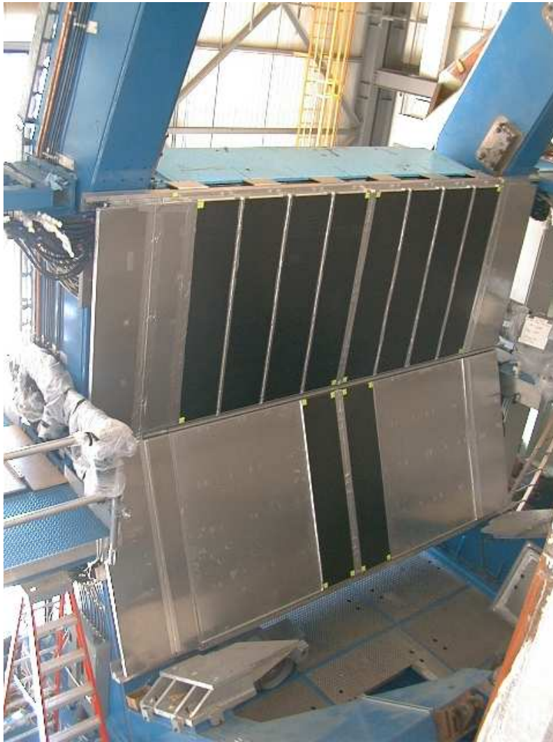
Figure B.1: The TOF detector system mounted on the PHENIX East Arm showing 10 panels of the detector.
