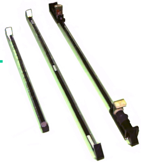
Slat: Plastic scintillator w. 2 PMT's
