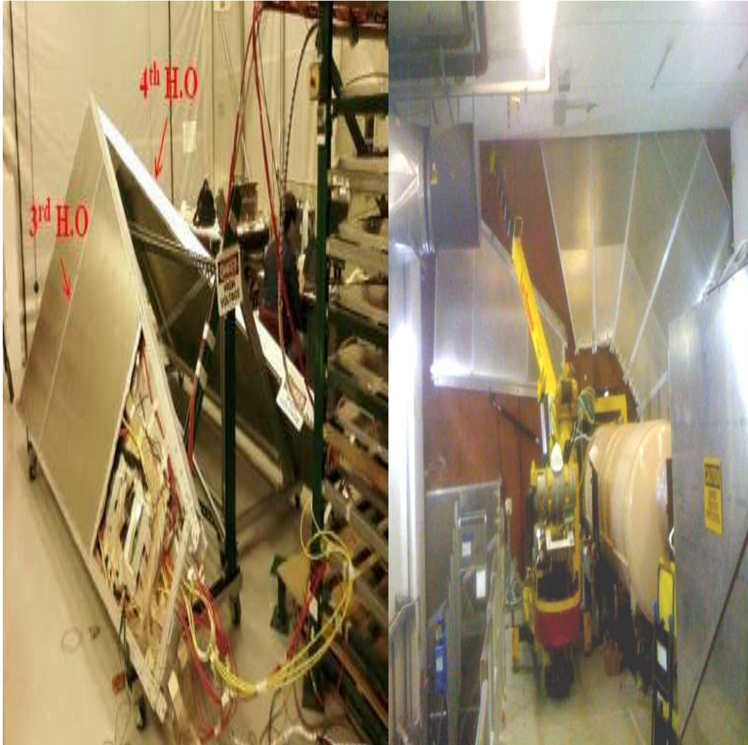
Figure 20: RPC-3 half octants being tested in RPC assembly laboratory at BNL, left and installation in progress at PHENIX, right.
