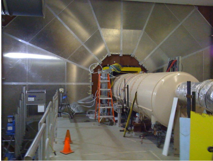
Figure 2: Installed RPC Detector for North muon trigger.
