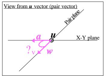
Reconstructed momentum vectors of e+e- pair made a plane(pair plane). If e+e- pairs come from photon conversion at R!=0, the plane is apparently made by B-field. Therefore, the plane is always perpendicular to B-field.
