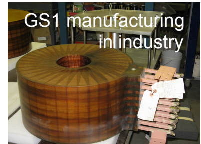
main solenoid manufacturing in SMD
