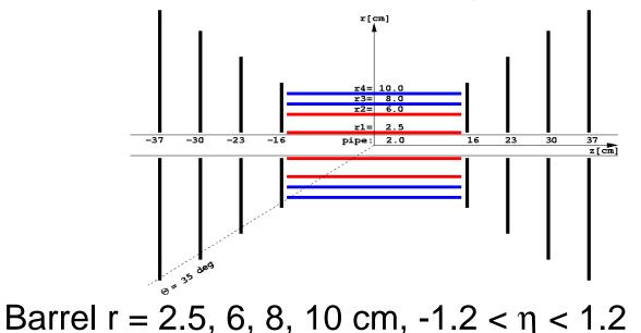
GEANT \* pixel barrels \* strip barrels \* pixel disks endcap, pixels 4 circular disks z=16, 23, 30, 37cm  $1.2 < |\eta| < 2.4$
