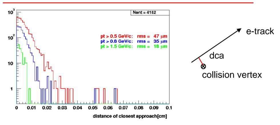
50µm x 425µm pixels, full multiple scattering dca resolution (electrons) < 50 µm less than  $c\tau$ , D<sup>0</sup>: 125µm D<sup>±</sup>: 317 µm
