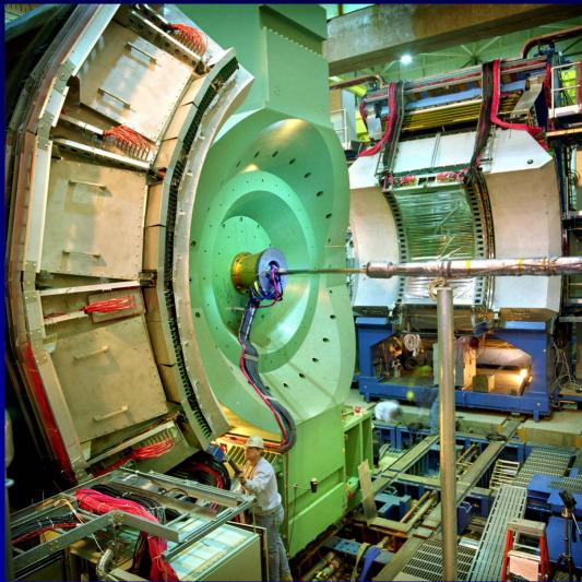
2 central spectrometers - Track charged particles and detect electromagnetic processes
