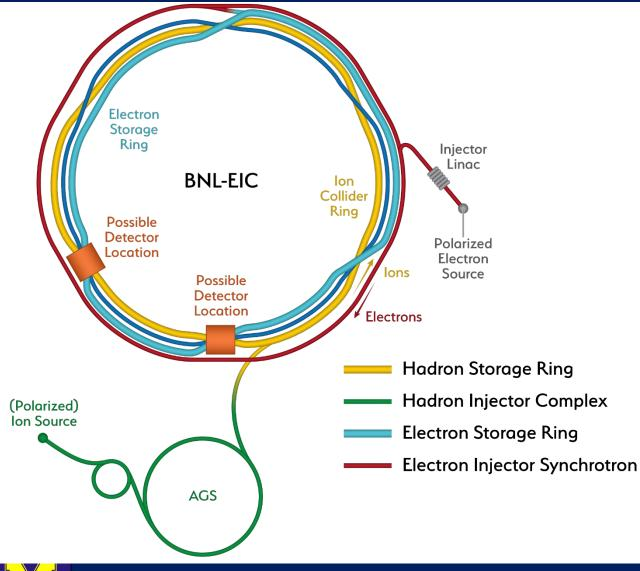
Add an electron injector complex with Rapid Cycling Synchrotron
