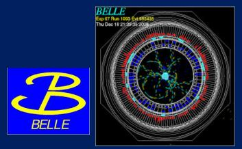
Tracks from electron-positron annihilation at the BELLE experiment, KEK, Japan
