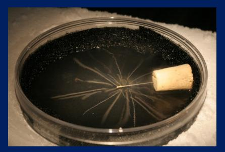
Make your own cloud chamber to observe cosmic rays! (Radioactive source shown here) -91% isopropyl alcohol -Dark felt -Small container with transparent lid -Dry ice
