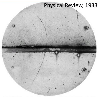
F16, 1. A 63 million volt positron  $(H_{\rho}=2,1\times10^{\circ} \text{ gauss-cm})$  passing through a 6 mm lead plate and emerging as a 23 million volt positron  $(H_{\rho}=7,5\times10^{\circ} \text{ gauss-cm})$ . The length of this latter path is at least ten times greater than the possible length of a proton path of this curvature.
