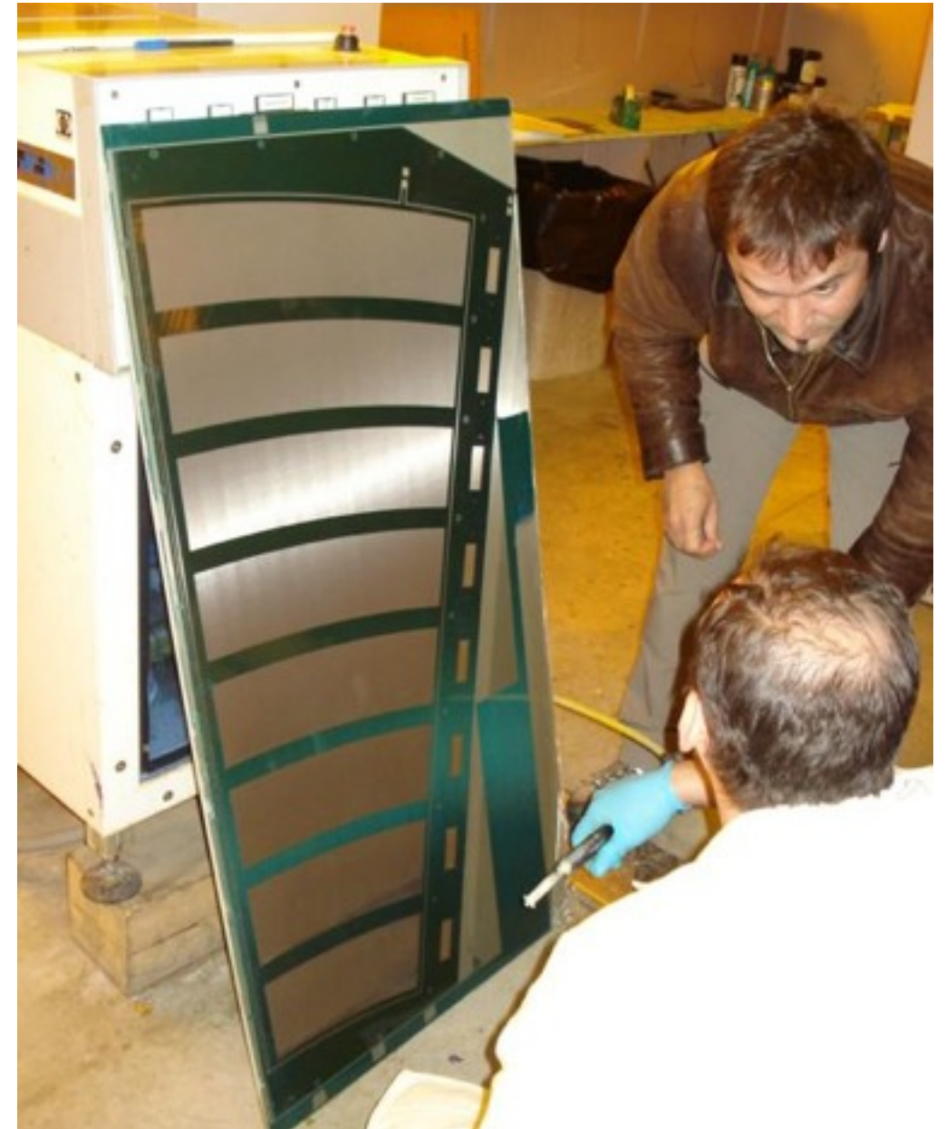
Chamber after pillar development but before curing
